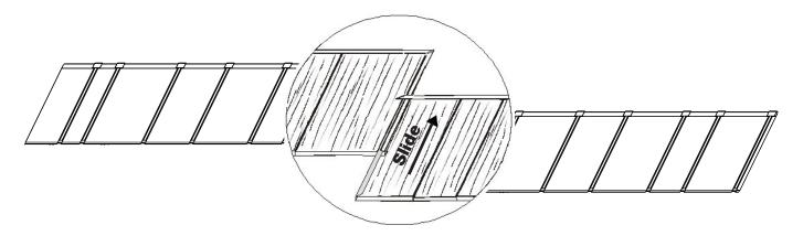
The siding is butted into the corner and nailed into place allowing approximately 1/16" space between the J-channel and the siding in warm weather installations and 1/8" space in cold weather installations. Using this common sense approach should insure a good appearance, and thus avoid unnecessary waves or buckles which could occur with temperature change.
